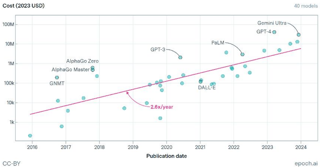
Amortized hardware and energy cost to train large-scale AI models over time EPOCH AI
